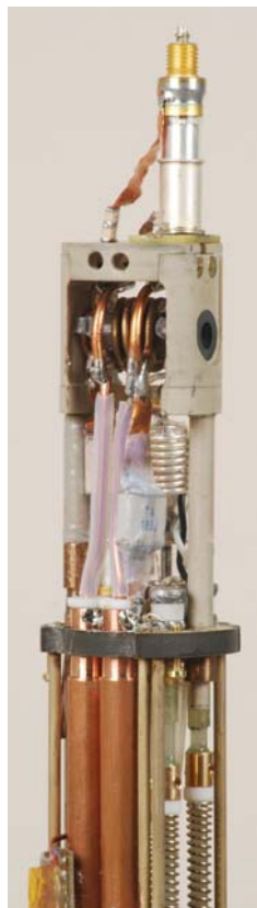
Figure 4 (above): Photo of completed prototype. The shield body tube (with the gradient coil) seats around the sample access so the entire probehead can be pressurized for increased power handling. The quartz variable capacitor extending from the top is the coarse-tune adjustment for the MF. Fine-tune adjustments for all three channels are accessible from the bottom.
