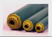
Thick wall rotors and Aurum, or Torlon caps are provided for **fastest spinning** and ease in packing.
