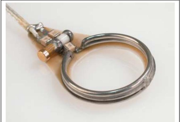
Figure 2. A 20 mm balanced T/R surface coil with heavy, magnetically compensated, parallel conductors. The thin acrylic coating over all the parts is not obvious, and the remote tune/match network, included in Figure 1, is not shown here but is at the remote end of the feed cable.
