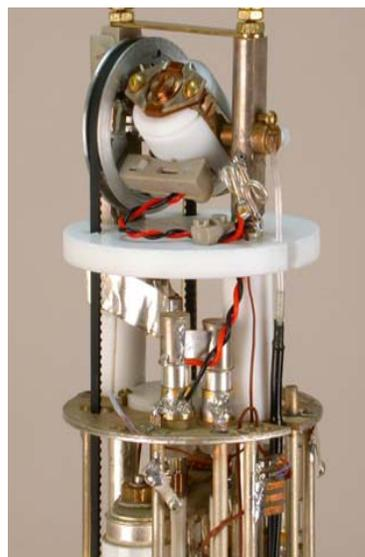
Figure 5. Photo of latest WB SAS probe using an XC4 spinner with novel approaches to rf leads and position feedback and encoding. A fused glass-fiber light pipe is visible coming in along the reorientation axis on the near side for optical spin-rate detection. The MF/LF lead connections on the opposite side are not visible in this view, but are handled in a way similar to commutator connections in some DC motors.
