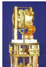
Figure 4. The LF/MF flex leads used on this earlier 600 MHz HXY SAS probe had to be replaced after ~50,000 flips.
