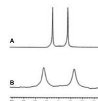
Figure 7. <sup>2</sup>H quadrupolar splitting for D<sub>2</sub>O in bicelles. A) spectrum for sample rotating at  $\theta=80^\circ$ . B) spectrum on rotating sample obtained with SAS from  $\theta=80^\circ$  to  $\theta=10^\circ$ , nt=8.
