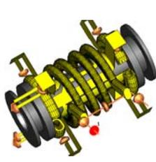
Figure 3. The <sup>1</sup>H XC and the LF/MF solenoid are shown here as simulated in CST MWS 5.0. The <sup>1</sup>H capacitors (8 for tuning, plus feed and balance) are represented by chamfered disks.
