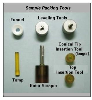
improved by mixing the material with a fine powder lacking interfering NMR signals. Tissues and fibers may spin better when packed wet. Some other materials should be dried and ground fine for best packing. A small funnel cup, a tamp, a rotor scraper, and sample leveling tools are provided to assist in packing rotors.
