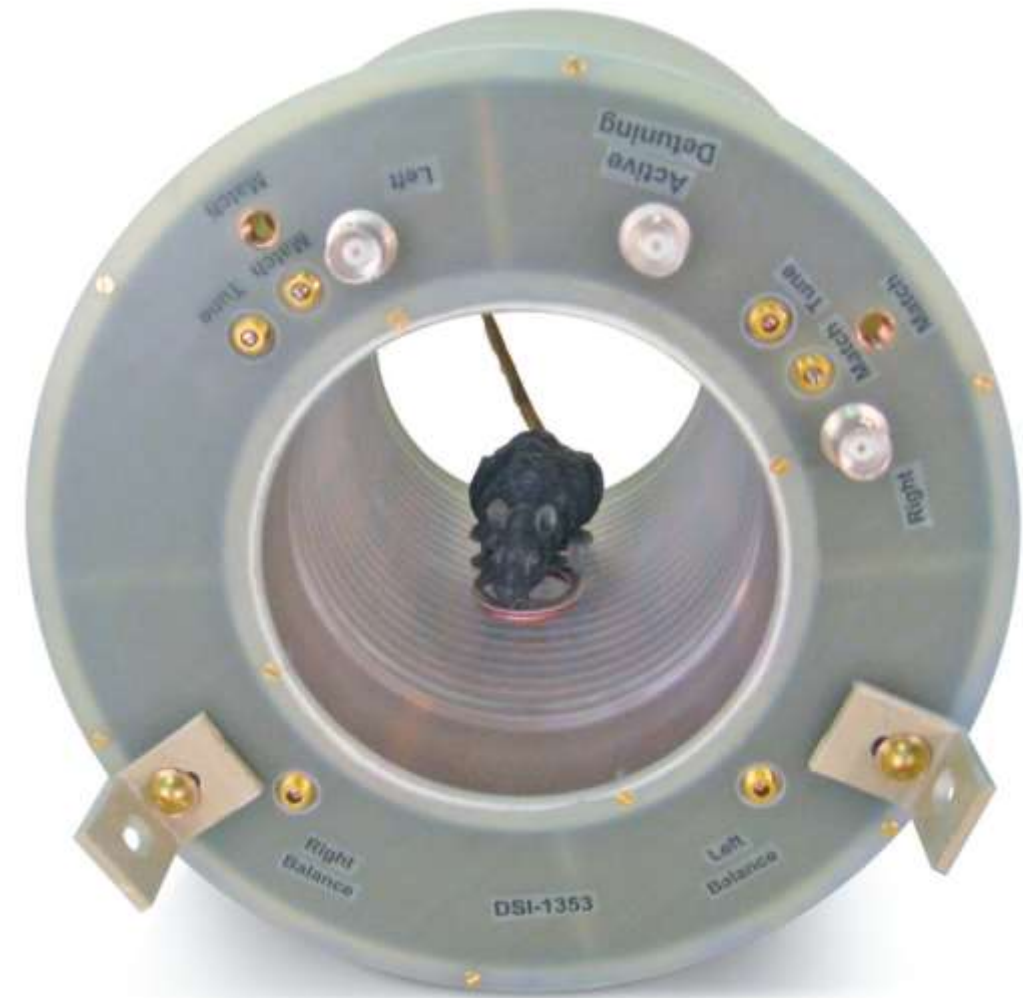
DOTY quadrature ^1\text{H} Litzcage module, with active detuning for surface coil receive.
