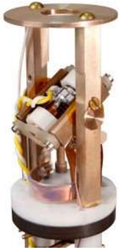
Doty 4 mm MAS with B_{\max} low-E ^1\text{H} coil.
