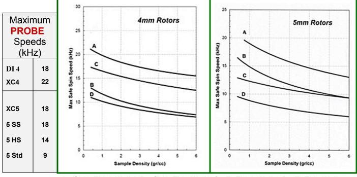
A - Si<sub>3</sub>N<sub>4</sub> Thick Wall | B - Si<sub>3</sub>N<sub>4</sub> Thin Wall | C - Zr Thick Wall | D - Zr Thin Wall
