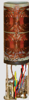
Vertical Bore MRI Probe with 3 axis gradients and a RF Litz or Litzcage coil
