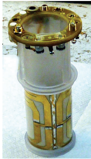
Inner multi-X Coil Outer ^1\text{H} - ^{19}\text{F} Coil Finished Coil, 15.2 T, ^1\text{H} - ^{19}\text{F} /X
