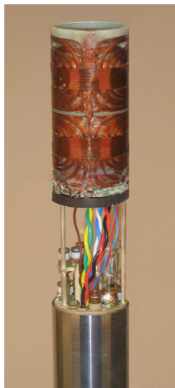
NB MRI Probe with 26-40 Gradients and RF
