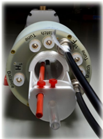
A Doty 9.4 T 32 mm ^1\text{H}/^{19}\text{F} Rat Brain Volume Coil. Shown with user incorporated animal bed.
