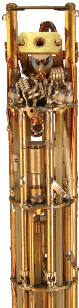
500 MHz, NB, H/F/X/Y 3 mm MAS Probe with 2 Broadband Channels
