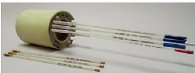
65 x 52 mm ^1\text{H}/\text{X} Dual Frequency Coils
