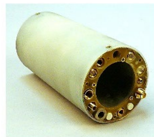
Finished Coil, 15.2 T, H-F/X
