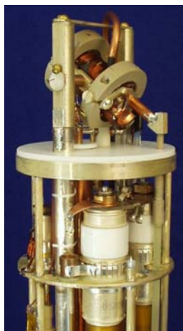
Figure 1 An MAS probe with a magic angle gradient coil (Doty Scientific, Inc.)
