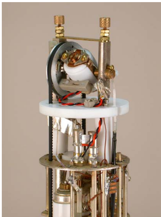
Figure 5 Photo of a WB SAS probe using an XC4 spinner. A fused glass-fiber light pipe is visible coming in along the reorientation axis on the near side for optical spin-rate detection. The MF/LF lead connections on the opposite side are not visible in this view, but are handled in a way similar to commutator connections in some DC motors.
