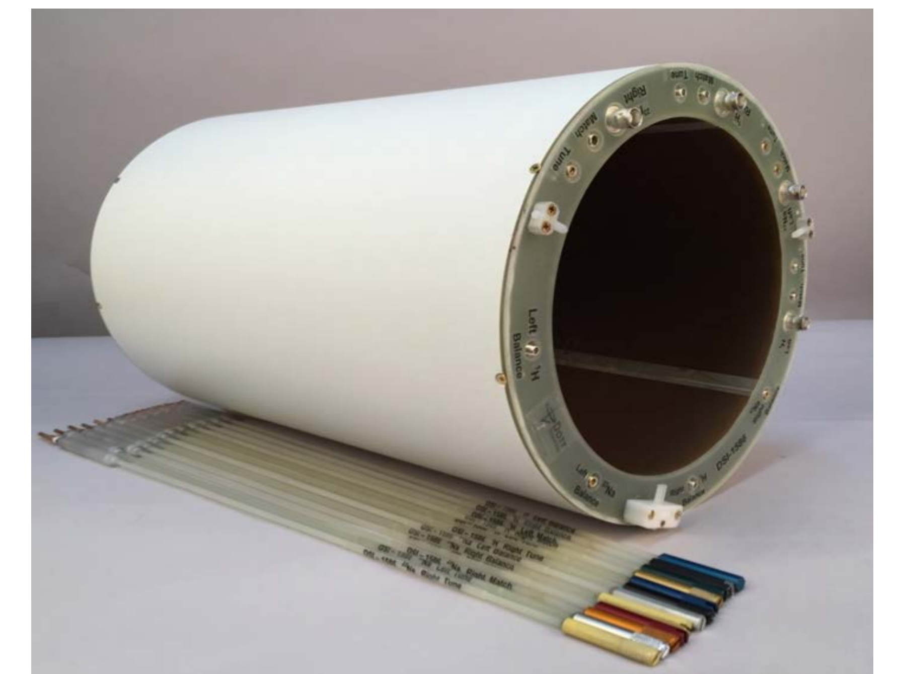
Fig. 6 4.7 T 1 H/ 23 Na volume coil. 20 cm ID x 20 cm RF rung length (25 cm OD).
