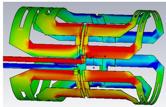
Fig 2. A perspective view of the inner CF2b multi-X coil showing  $I_z$  at 100 MHz.
