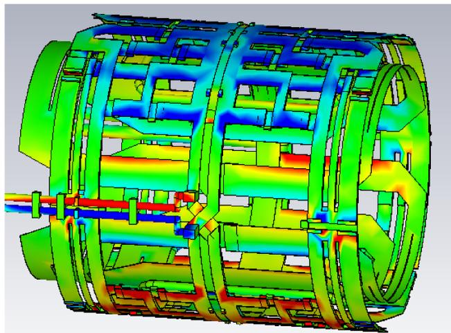
Fig 1. Foil patterns showing  $I_z$  on the coil surfaces when the outer coil is driven at 650 MHz.
