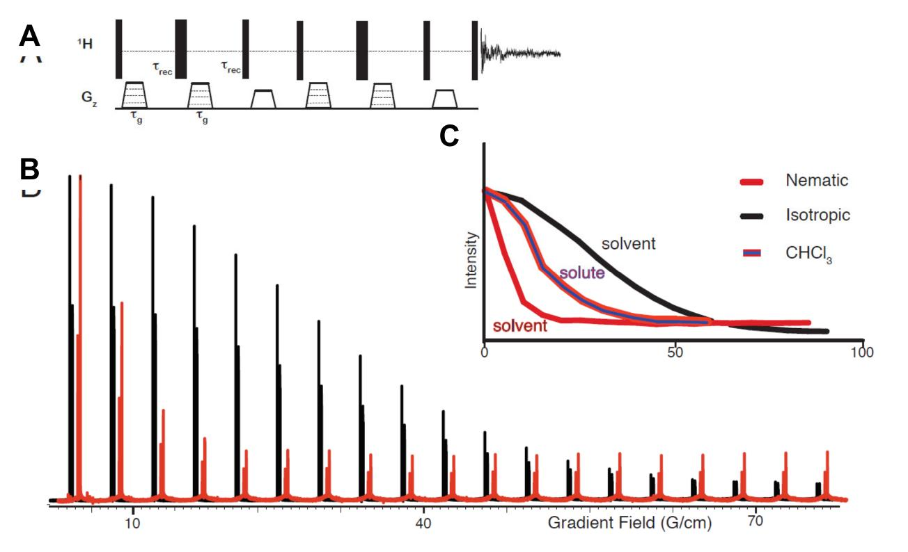
A) Stimulated echo pulse sequence for PFG-diffusion NMR study of a nematic liquid crystal 5CB under MAS. B) Array of <sup>1</sup>H spectra recorded under 7 kHz MAS with varying gradient strength. Black and red colors indicate isotropic and nematic phase of 5CB. C) Graphical demonstration of signal decay for solvent (5CB) and the solute (CHCl<sub>3</sub>).
