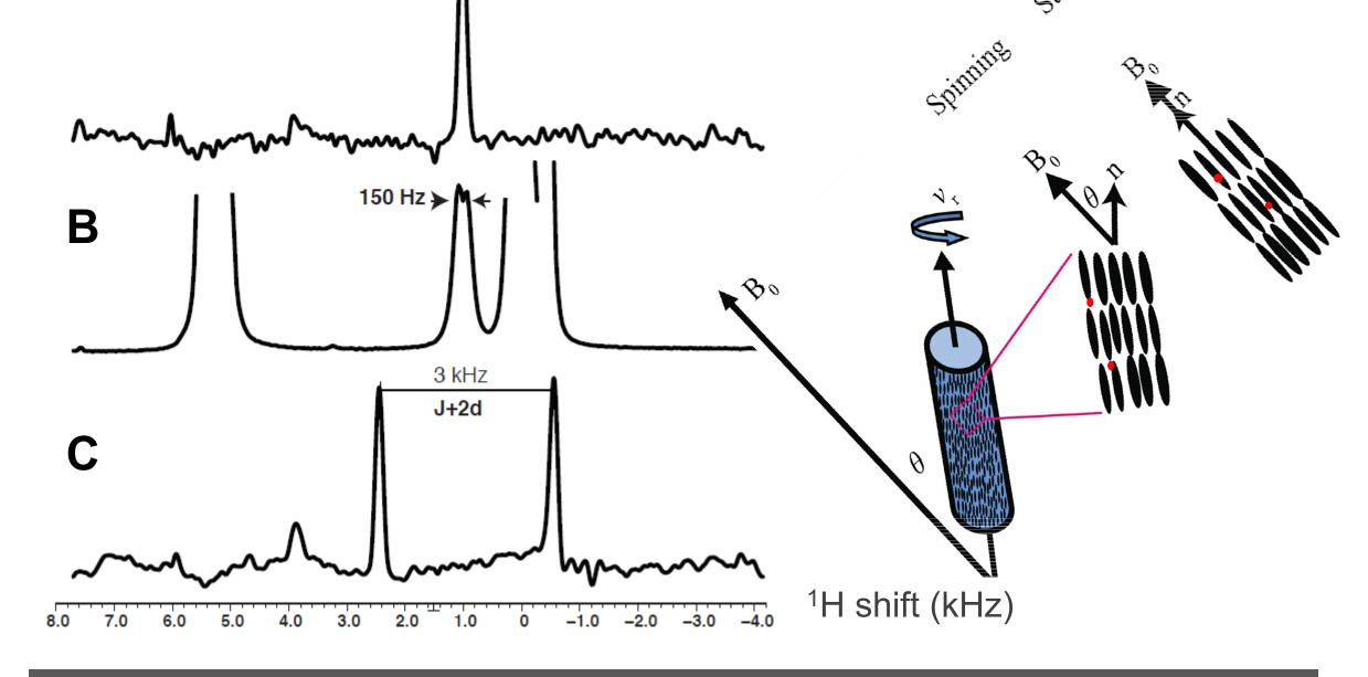
300 MHz <sup>1</sup>H signal of chloroform in nematic 5CB. A) <sup>13</sup>C decoupled 10 ms spin echo signal obtained under MAS. B) 1ms echo signal under MAS and no <sup>13</sup>C decoupling applied. C) <sup>13</sup>C coupled 1 ms echo signal under stationary conditions. 3 kHz splitting in C accounts for sum of  $J_{CH}$ -coupling and twice  $d_{CH}$ -coupling.
