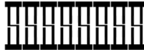
Figure 1. The first-surface of the litzcage pattern is shown. (The other surface on the laminate completes the central crossovers.) The pattern wraps around a cylinder aligned with B 0 (vertical in this view) and generates a transverse CP B 1 .
